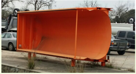
Examples of truncated cone beds. It's like dumping out of the top end of a funnel.
